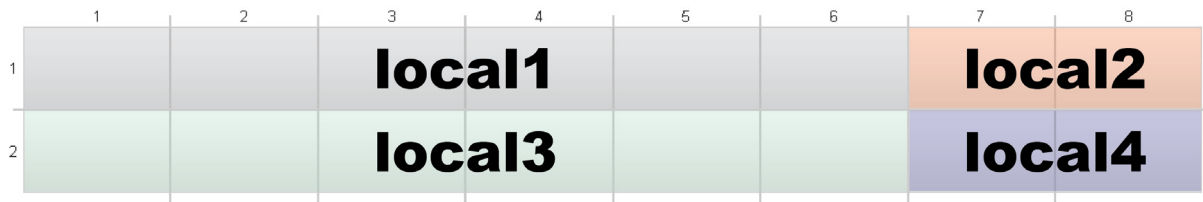
Figure 4-3 Window Locales in a 2 × 8, 2K/HD Wall
